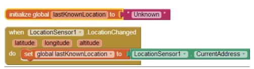
**Figure 4-9.** Recording the phone's location in a variable each time the GPS location is sensed
