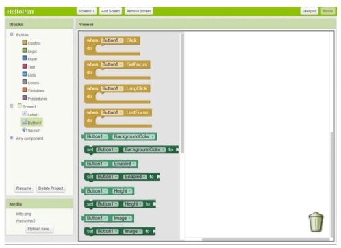
Figure 1-9. Clicking Button1 shows the component's blocks
